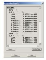
Figure 19-15. The **Integration** dialog and the integration results for calculating the lift and drag for the data shown in Figure 19-14.
