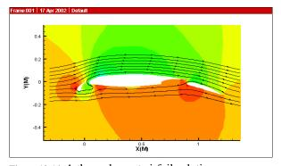
Figure 19-14. A three element airfoil solution.
