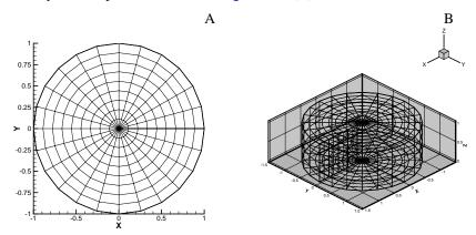
Figure 18-7. (A) A 2D circular zone (B) A 3D circular zone.
