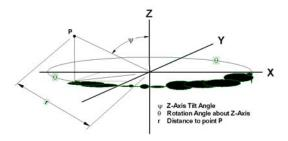
Figure 18-6. Three-dimensional angles of rotation.
