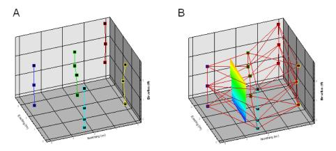
Figure 29-7. Tetra-Grid example. The original well data (A), tetrahedral zone from the well data (B)
